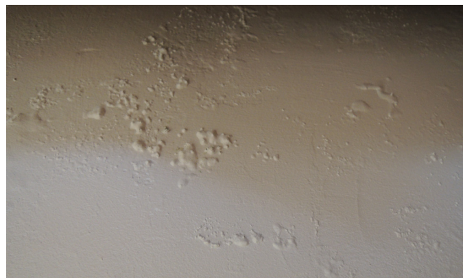
Typical failure of acrylic coatings.
